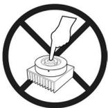
**The CTM dome diffuser is fragile. Avoid touching the dome diffuser during handling and assembly.**
